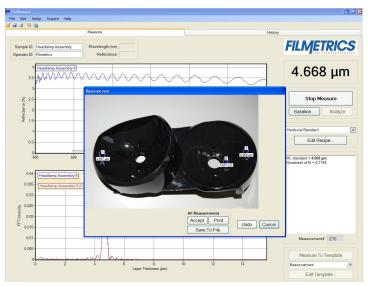
The user can import an image of the sample into the software and define measurement points.
